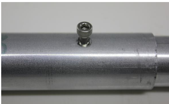
Screw fits into recessed hole - face up
