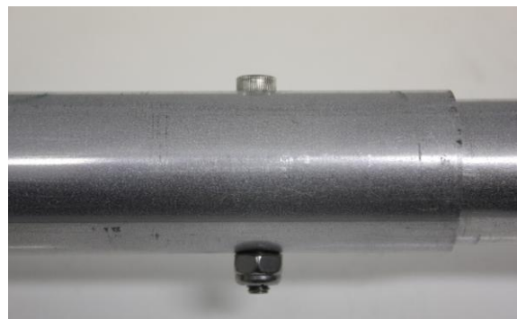
Nylon Nut placed on opposite end - face down
