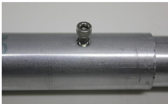
Screw fits into recessed hole - face up
