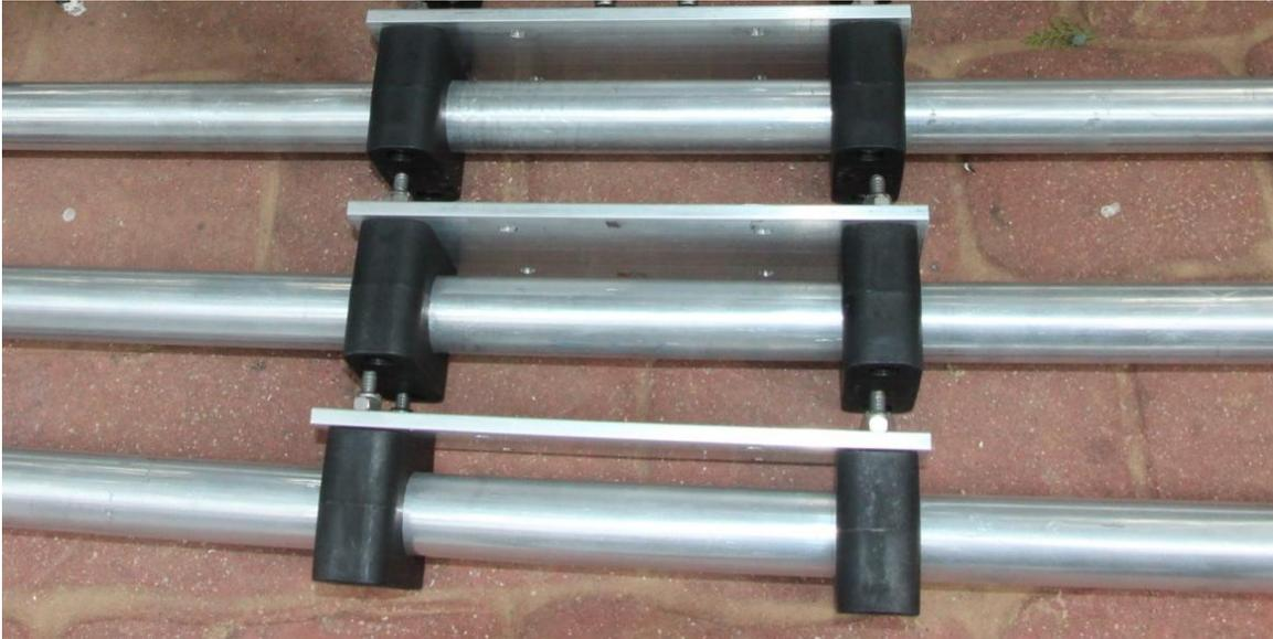
*20M center sections mounted on element plates*
