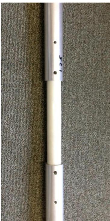
The fiberglass rod has 4 holes, two of which are 1/4" holes, and two of which are #10. The #10 holes are the outside holes from the center and are used for the mechanical mounting of the tubing to the fiberglass. The 1/4" holes are used for mounting the coil.
