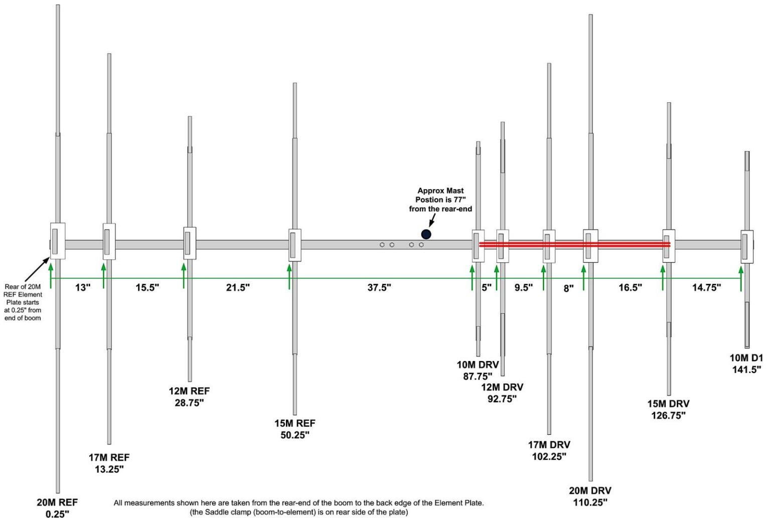
**\*\* All measurements shown here are taken from the reflector-end of the boom to the back-edge of the Element Plate.**
