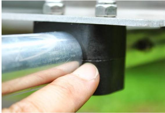
Make sure to center the tubing exactly at the mid-point of the plate.
