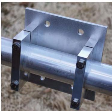
*Boom to Mast Plate attached to Boom*
