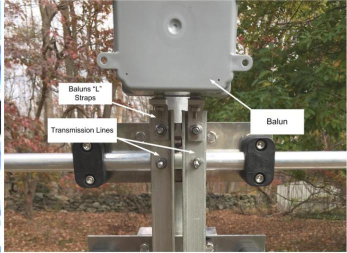
The JK NAVASSA-5 is delivered without a balun. We recommend a 1:1 current balun since the antenna is designed to be fed with a 50 Ohm balanced source, bringing the antenna to true optimum performance.
