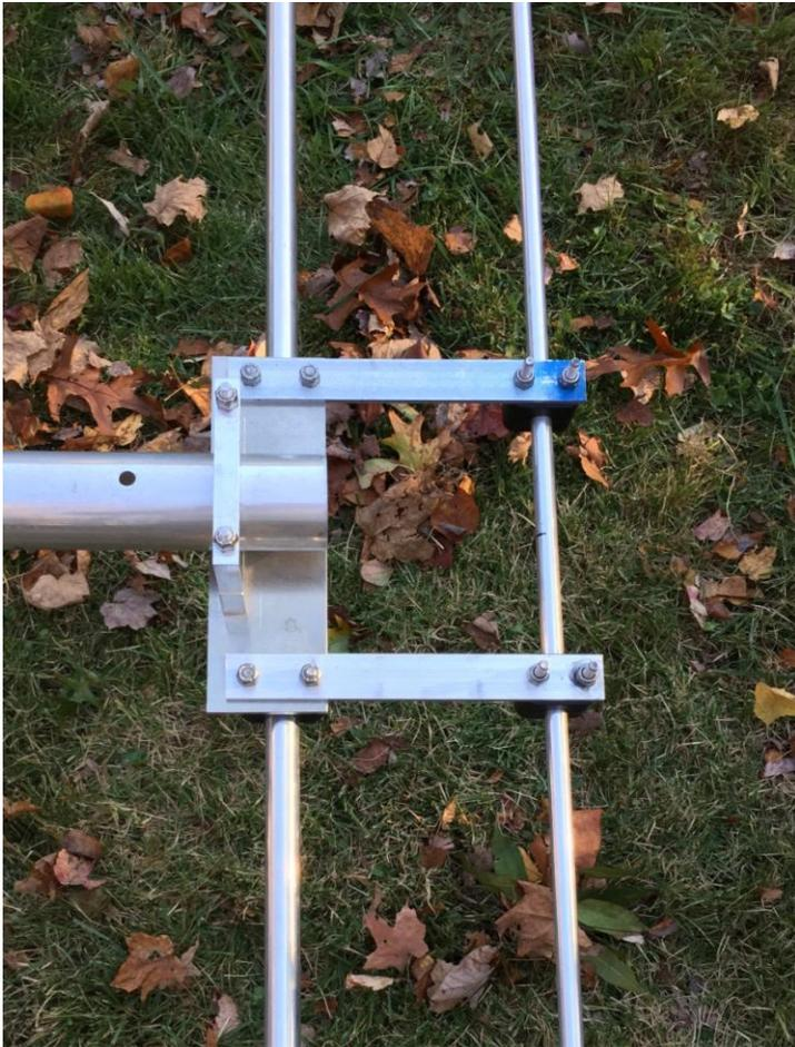
**The 6M elements are NOT mounted on the boom** - the 6M DRV element is mounted onto the Boom to Element Plate of the 15M DRV Element, and the 6M D1 element is mounted onto the Boom to Element Plate of the 10M D1, using special **Element Brackets**.
