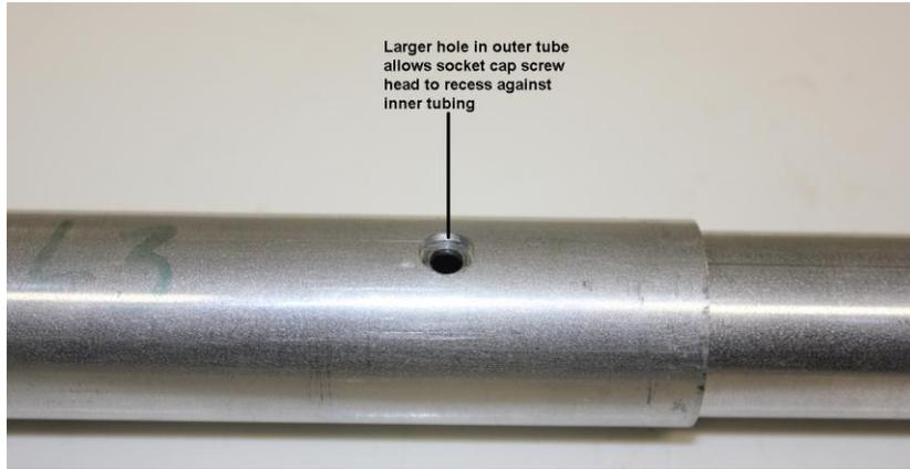
Each tube has one larger, counterbored hole drilled on one end, on one side. **The side of the tube with the counterbored hole is ALWAYS the outer tube of a joint, with the smaller outer-diameter tube sleeved inside.**
