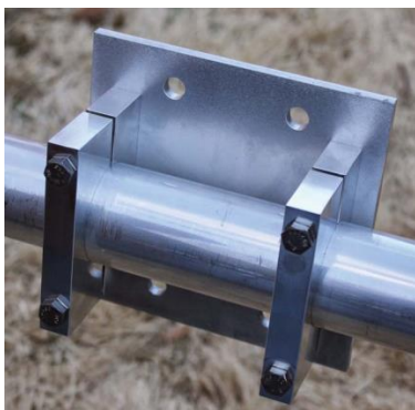
Boom to Mast Plate attached to Boom
