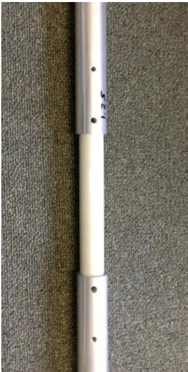
The fiberglass rod has 4 holes, which are 1/4" holes. The outside holes from the center and are used for the mechanical mounting of the tubing to the fiberglass. The inside holes are used for mounting the coil using the Full Thread screws.
