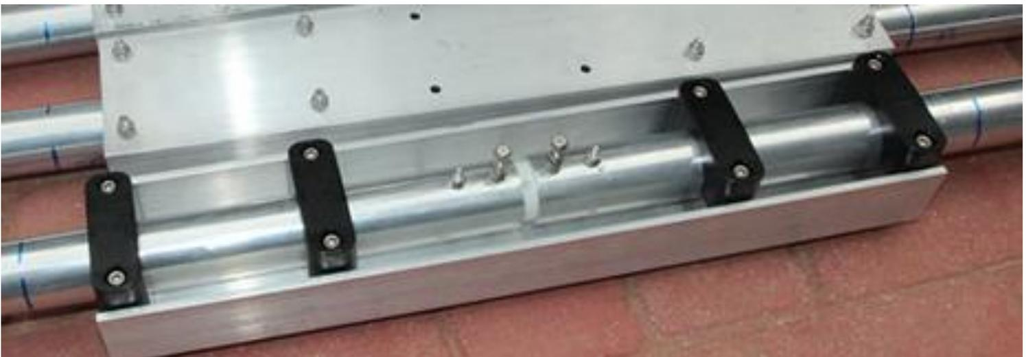
*40M center sections mounted on element channels*
