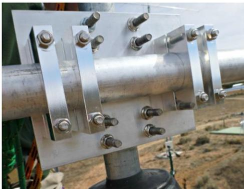
*Boom to Mast Plate attached to Boom
