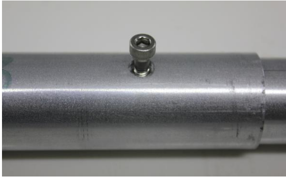
Screw fits into recessed hole - face up
