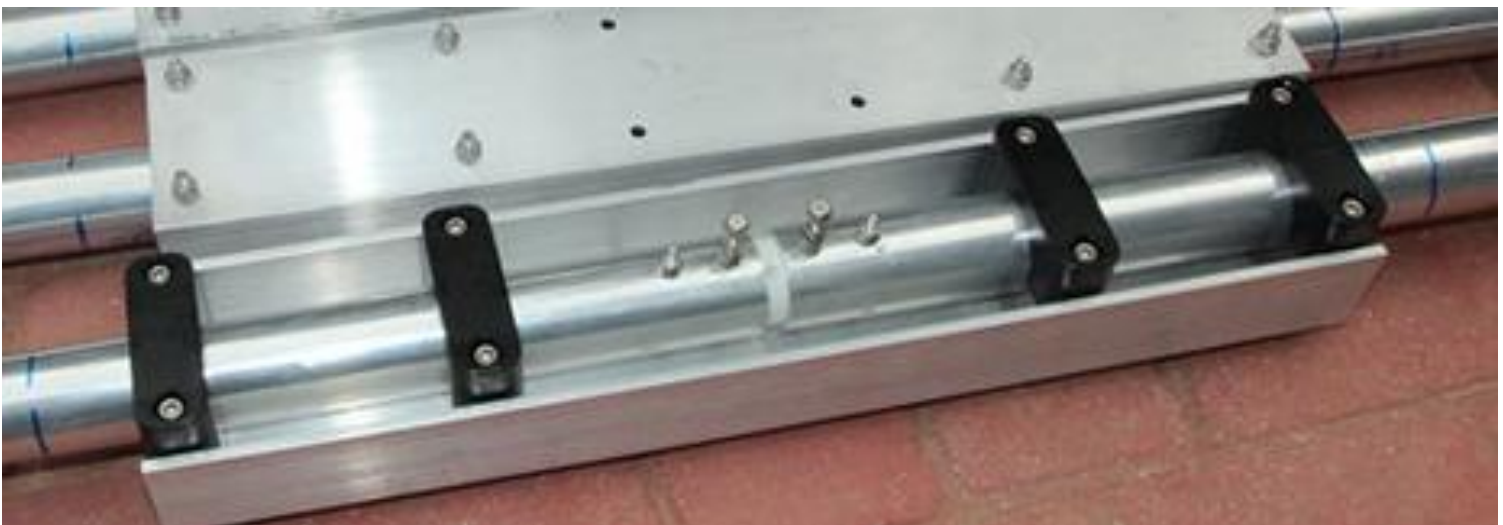
40M center sections mounted on element channels
