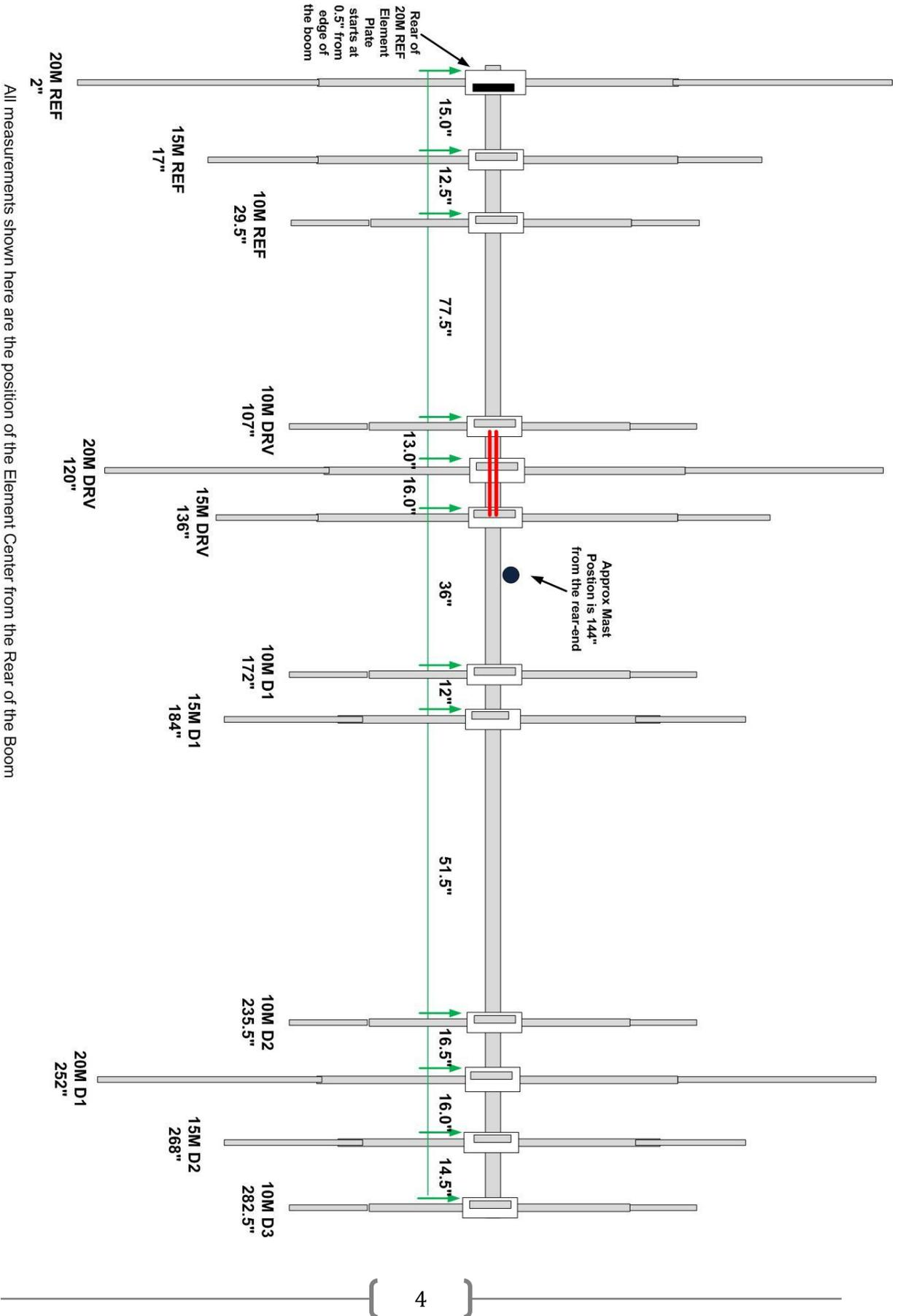
Recommended assembly method: Mount a short (5 foot tall) temporary mast into the ground. Mount the **Boom to Mast Plate** onto the short mast with the U-bolts from the **Mast to Plate Kit** and continue with assembly of the antenna. Once finished, remove the U-bolts and re-attach the assembled antenna on your tower.
