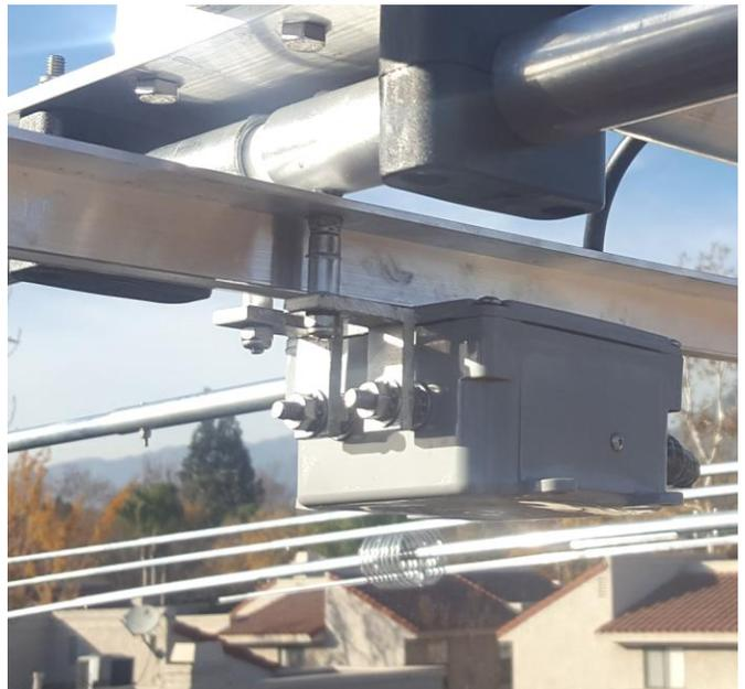
The JK MIDTRI is delivered without a balun. We recommend a 1:1 current balun since the antenna is designed to be fed with a 50 Ohm balanced source, bringing the antenna to true optimum performance.
