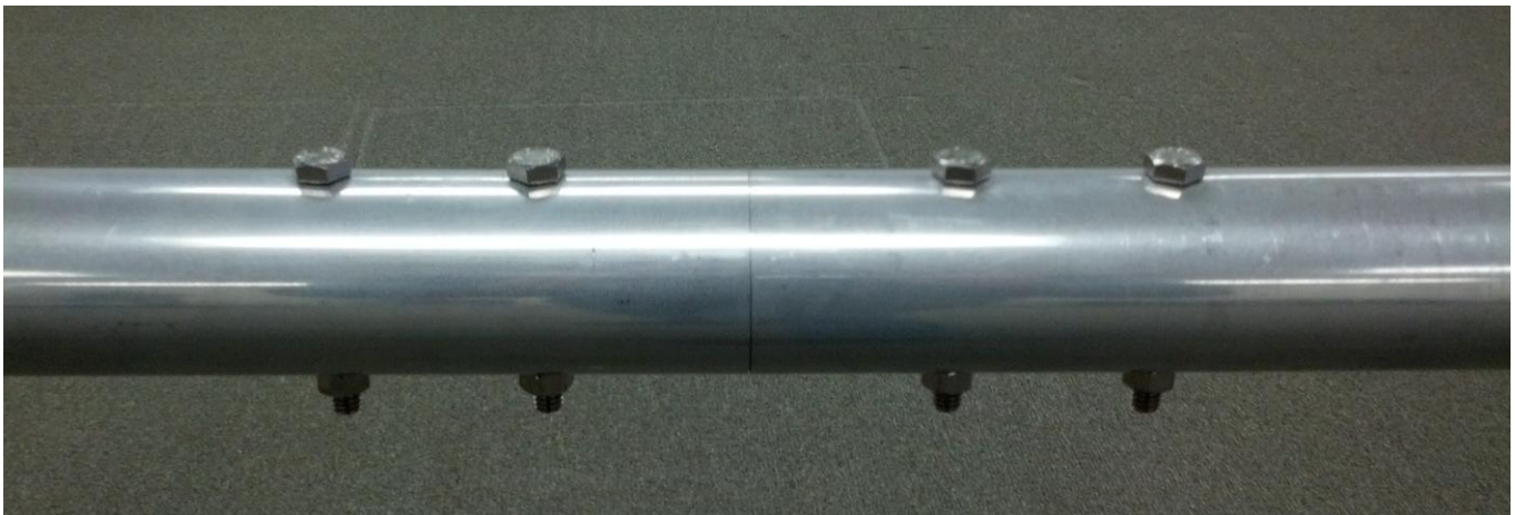
Assembled Boom Joint
